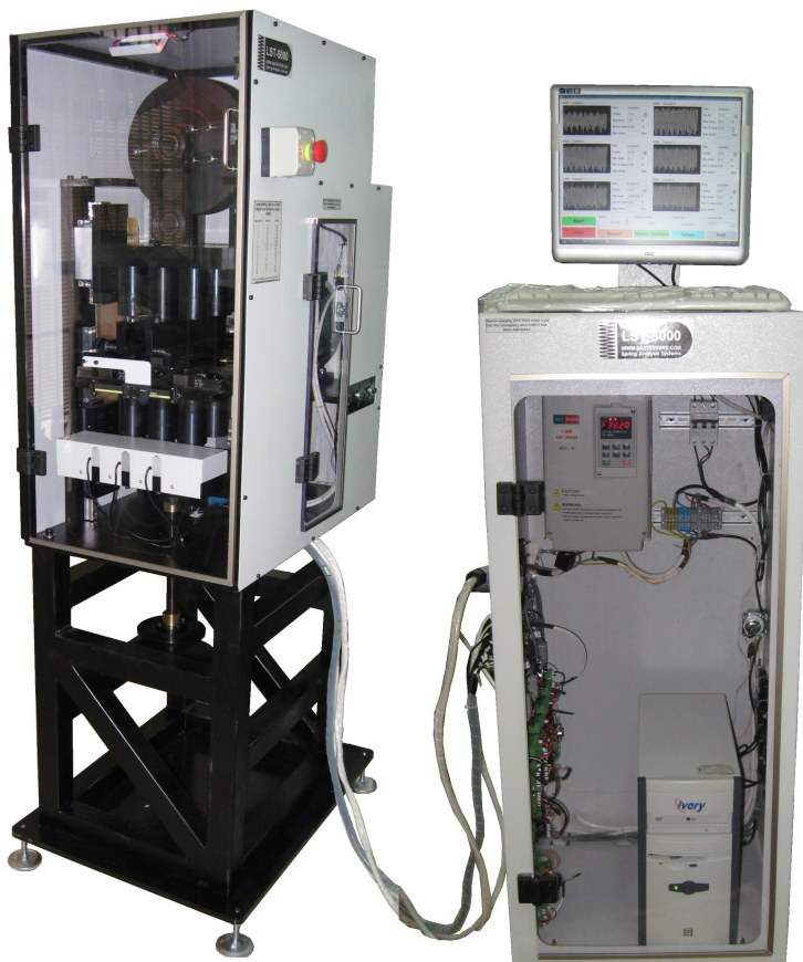
LST5000-PC shown with control cabinet and 6 load cell stations
